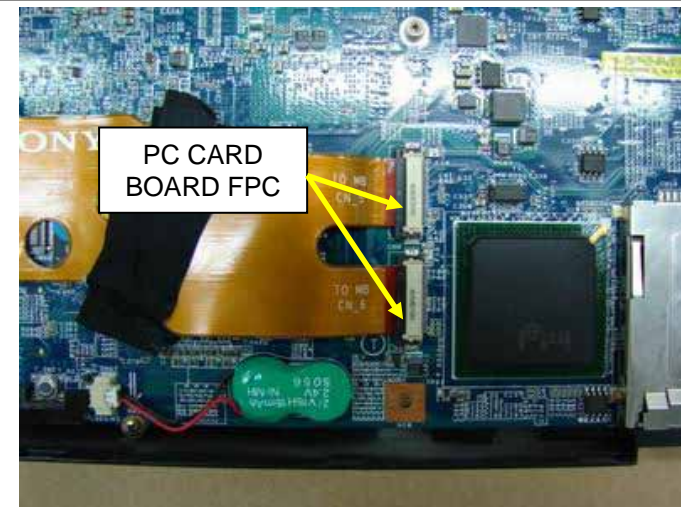
DISCONNECT THE TWO CONNECTORS ON THE PC CARD BOARD FPC AND REMOVE THE FPC
